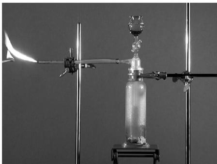
Figure 1. Demonstration experiment "carbide lamp": Calcium carbide reacts with water by forming the combustible gas ethyne (in spite of its high positive  $\mu$  value) because the chemical potentials of the reactants together exceed those of the combined products:
